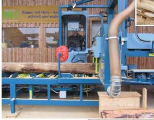
Vision Tilt actively corrects the saw band's position on the band wheel, which not only minimises wear but also improves sawing accuracy.
