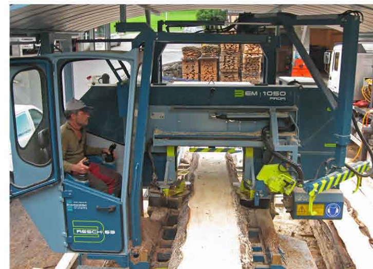
Optimal overview from the driving cab of the saw blade guide, double precutter, cross cutter, plank remover and ensures a constant quality control of the sawn timber
