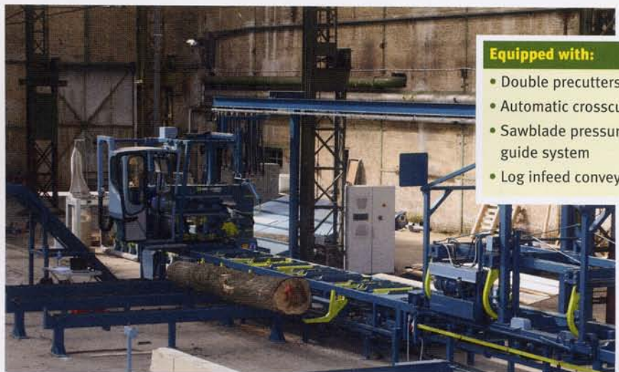
Complete stationary bandsaw line ES 1050 PROFI with automatic sorting system
