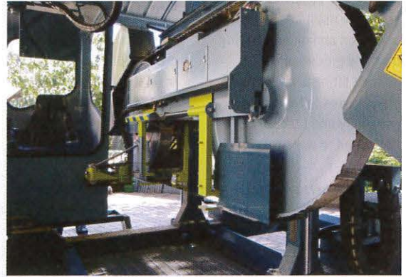
Fast sawblade change. The protective housing is opened hydraulically.
