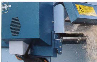
No suction unit, the sawdust collection box empties itself at the final position
