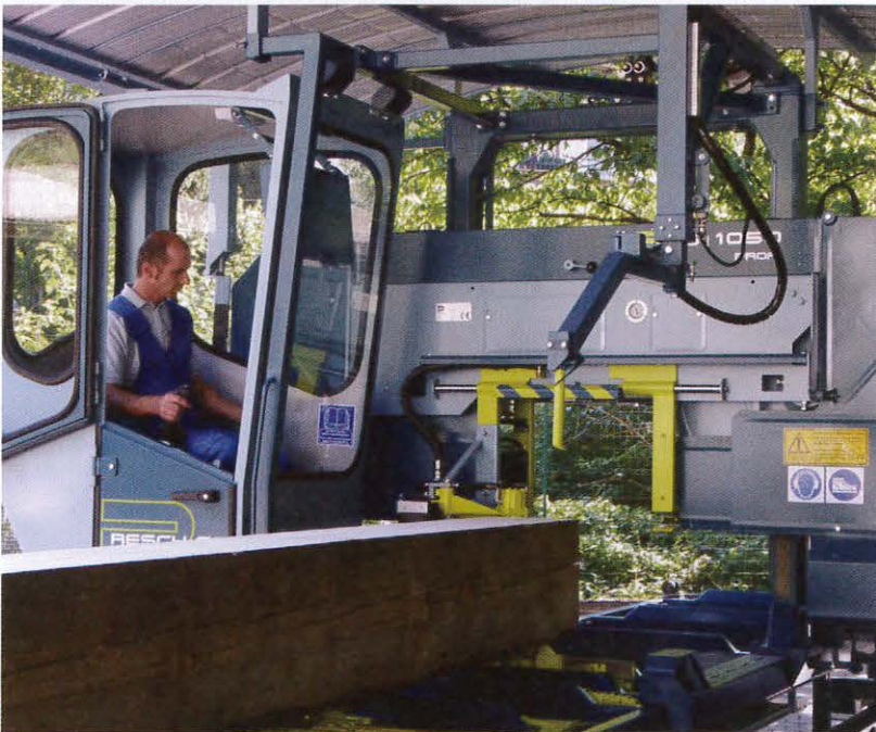
Owner Christoph Lunger shows the new stationary bandsaw type ES 1050 PROFI. The travelling cab ensures the operator has a perfect view of the timber and optimal visibility of the pre-cutters, crosscutter and sawblade pressure guide.
