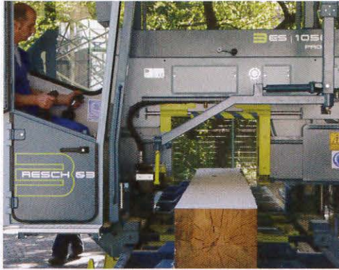
Automatic board remover. To cut quality goods, it is important that the operator after each cut can see the wood quality. The board remover can take off on the side each board when travelling backwards.
