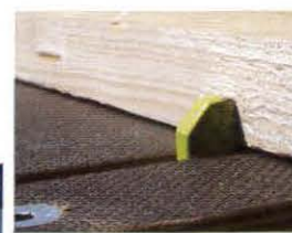
Lateral stops can be adjusted from 3 to 16 cm
