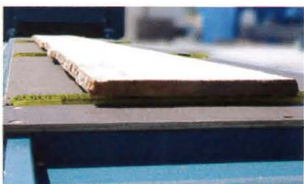
Cross chains for adjusting and ejection
