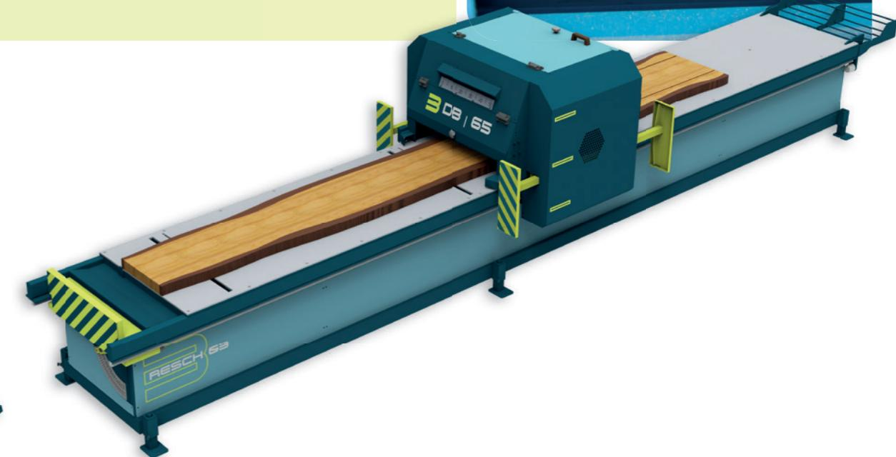
**High precision:** The plank remains on the table, while the sawhead travels back and forth. Two pressure rollers in front and behind of the saw blades hold the wood in place with downward pressure during the cutting process. This manufacturing process is unique to the market and guarantees an exact, parallel and straight cut.
