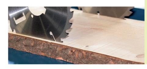
**High precision:** The plank remains on the table, while the sawhead travels back and forth. Two pressure rollers in front and behind of the saw blades hold the wood in place with downward pressure during the cutting process. This manufacturing process is unique to the market and guarantees an exact, parallel and straight cut.
