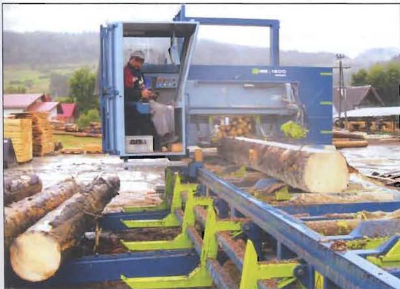
(Left) No part of Europe is exempt from inclement weather and this Eastern European customer no doubt appreciates the benefit of a fully insulated protective operator cabin. The Resch & 3 1200 Profi can cut timber with a diameter of up to 1.5 metres. (Right) Where visual monitoring of individual board quality is necessary during the milling process a board removal system can be fitted. Boards and slabs are automatically removed during the return travel phase and placed alongside the machine. This allows the operator to inspect the exposed surface of the timber before the next cut begins.
