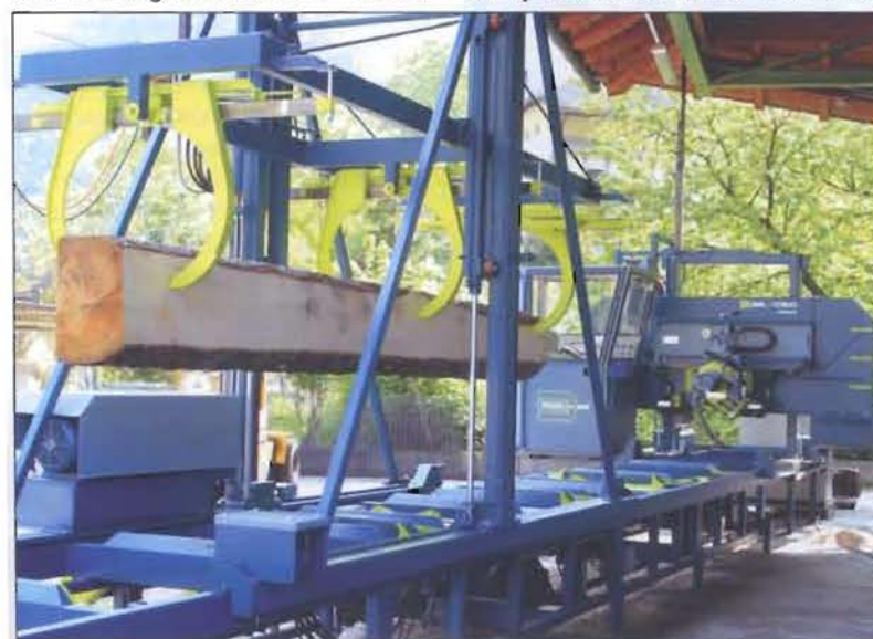
For static systems the Italian manufacturer can supply the three-tonged gripper carriage. The operator, from the cabin, is able to remove and separate slabs, balks or boards (singly or in stacks) clear of the sawing area.
